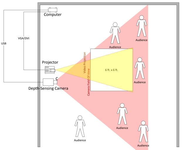
Projector are attached to ceiling or wall at a height of ~12'-15'. A wall attachment will require the projector and camera to be angled and special calibration performed. Both devices are attached to a computer which manages both computer vision and video sequencing.
